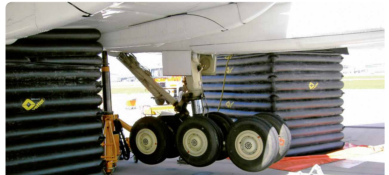
Aircraft Lifting Bags - quick and secure recovery
