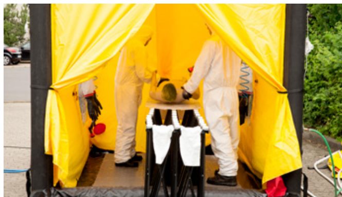
Double decon showers are particularly suitable for the decontamination of lying injured persons.
